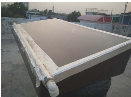
Figure 2: Constructed Solar Still
